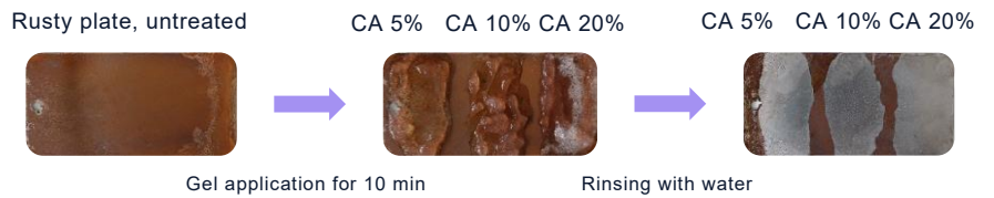
Figure 2: Results from performance testing of gel formulation containing different concentrations of citric acid (CA), after ten minutes treatment
