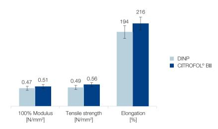
Fig. 1: Tensile strength - 100% Modulus - Elongation at break
