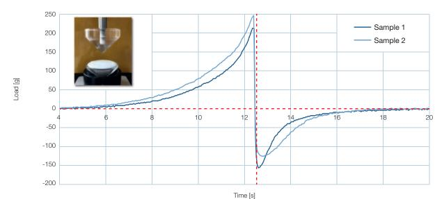
Figure 2: Compression test of two samples with significantly different texture profiles. Sample one is firmer and more adhesive than sample two.
