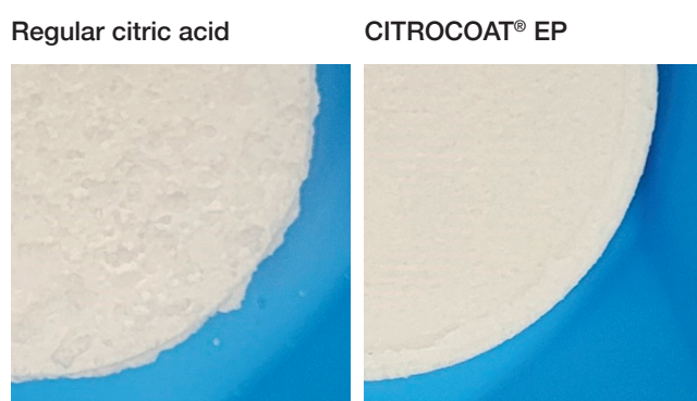
Figure 4: Visual assessment of effervescent tablets after being stored open for 88 days under harsh conditions (30°C, 60% relative humidity), with foaming and caking visible for regular citric acid tablets and no change visible for tablets with CITROCOAT® EP
