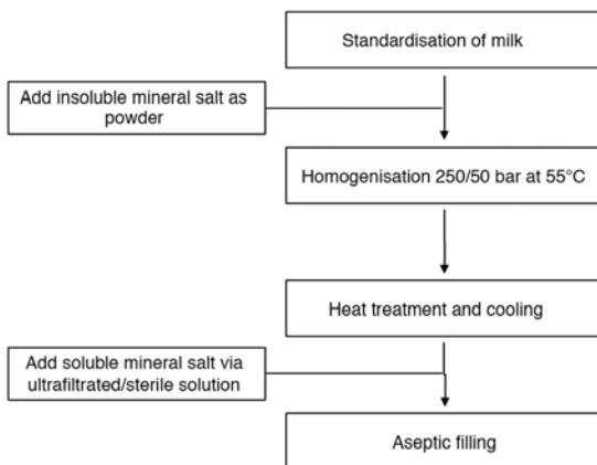
Fig. 1: Process flow chart for fortified UHT milk
