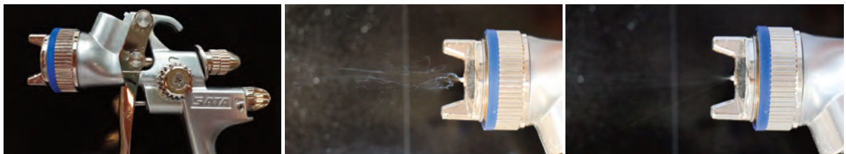
Figure 5: Spray gun (left) as well as a poorly (middle) and a well-defined (right) spray ‘fan’
