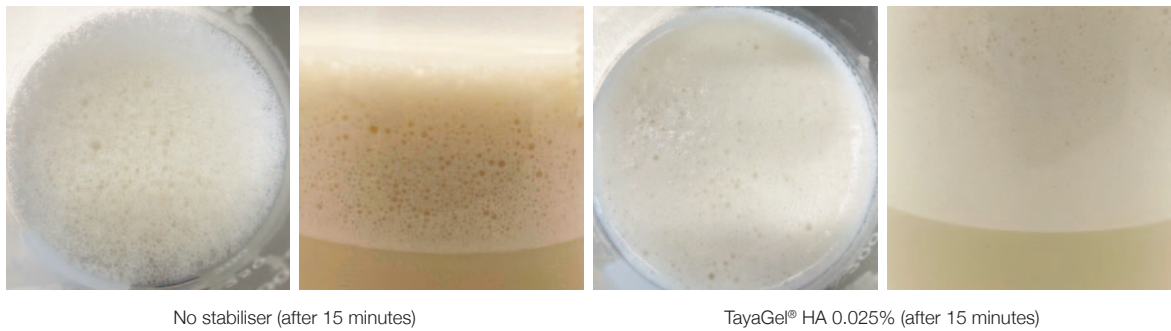
Figure 1: Foam appearance without (left) and with (right) TayaGel® HA as a stabiliser, 15 minutes after heating and frothing
