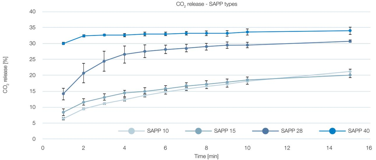
Figure 1: CO<sub>2</sub> release (%) of four different SAPP types.
