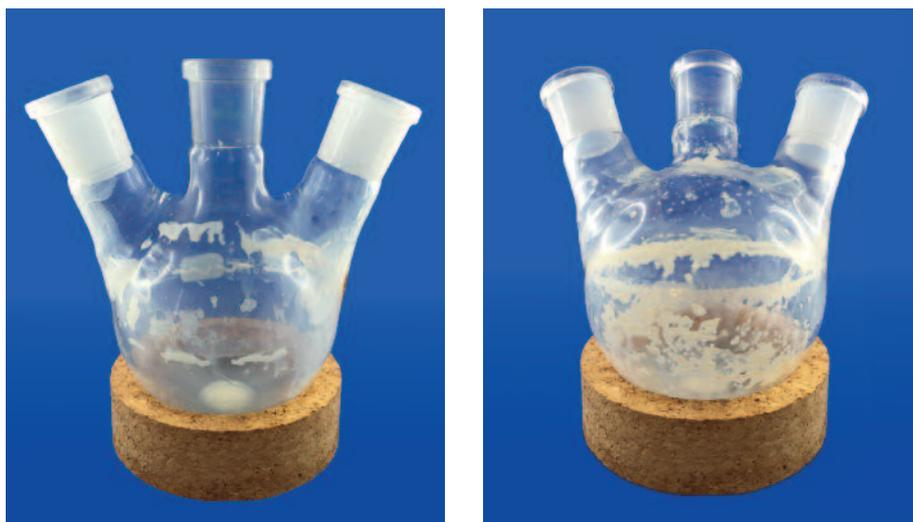
**Table 2: Overview of samples prepared and level of fouling in lab trials. 0 = no fouling, 1 = thin fouling layer, 2 = medium fouling layer, 3 = severe fouling incl. burnt particles.**
